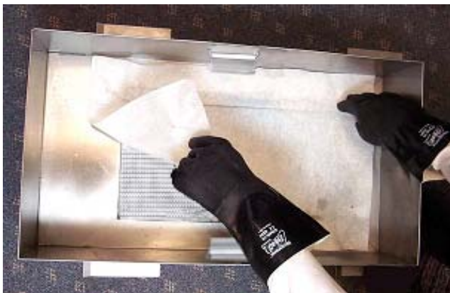
Remove and discard old filter paper.
