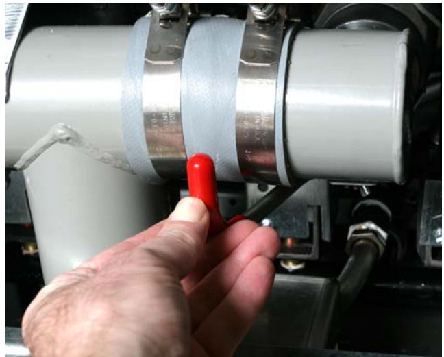
Push red drain valve handle from left (closed) to right (open). Oil will start to drain into filter pan.
