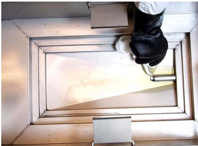
Clean filter pan and all pan components. Dry all parts completely before reassembly.
