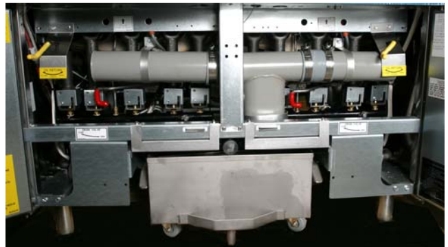
Pushing filter pan back into cabinet. Filter is ready for operation.
