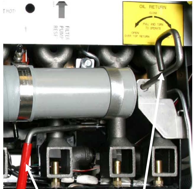
Drain valve handle (red).
